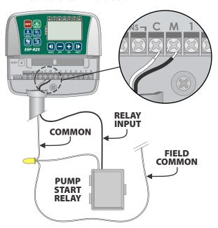
Connect the common wire from the pump start relay to the COMMON (C) terminal.
