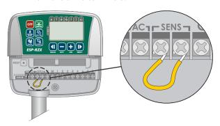
Connect both Rain Sensor wires to the SENS terminals.
