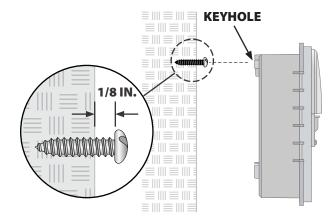
Drive a second mounting screw through the open hole inside the wiring bay and into the wall. Verify that the unit is fastened securely to the wall.
