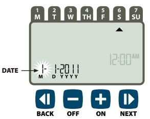
Press + or - to set the hour (ensuring that AM/ PM setting is correct); then press NEXT to select and set the minutes.
