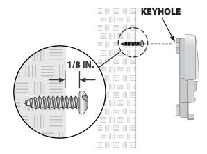
Drive a second mounting screw through the open hole inside the wiring bay and into the wall. Verify that the unit is fastened securely to the wall.
