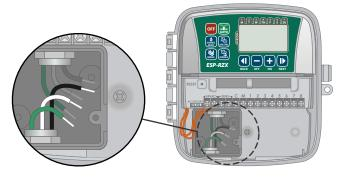
▶ Using the provided wire nuts, connect the external power source wires (two power and one ground) to the transformer connection wires inside the wiring compartment.
