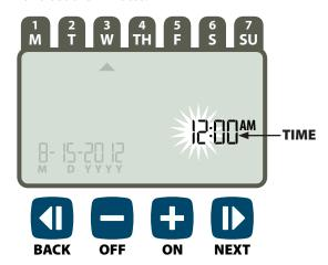
**NOTE:** Two AAA batteries can be installed to retain date and time in the event of a power outage. See "Install Batteries" for details.
